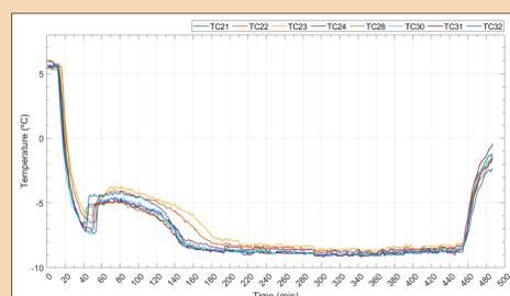
Evolution of the inlet, outlet and tank temperatures
