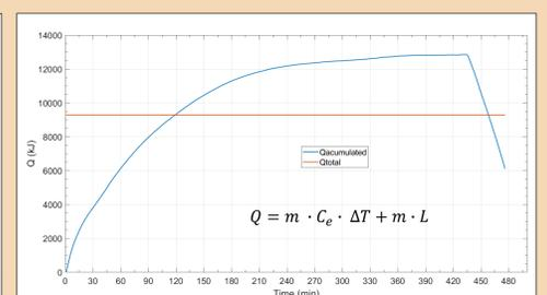
Evolution of the heat stored during loading and unloading as a function of the temperature
