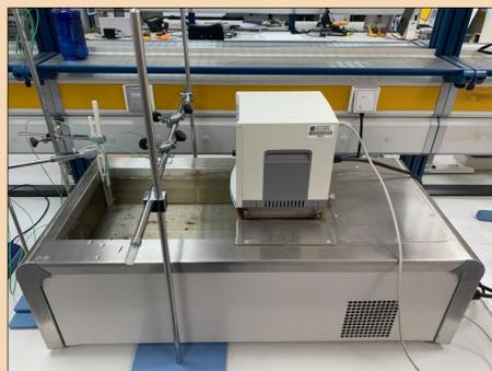
Cooling prototype of the cold storage tank
